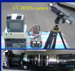
UV-HDTV camera (UV sensitive I.I.-HDTV camera, above) and I.I.-HDTV camera with grism (Direct vision grating, below).
